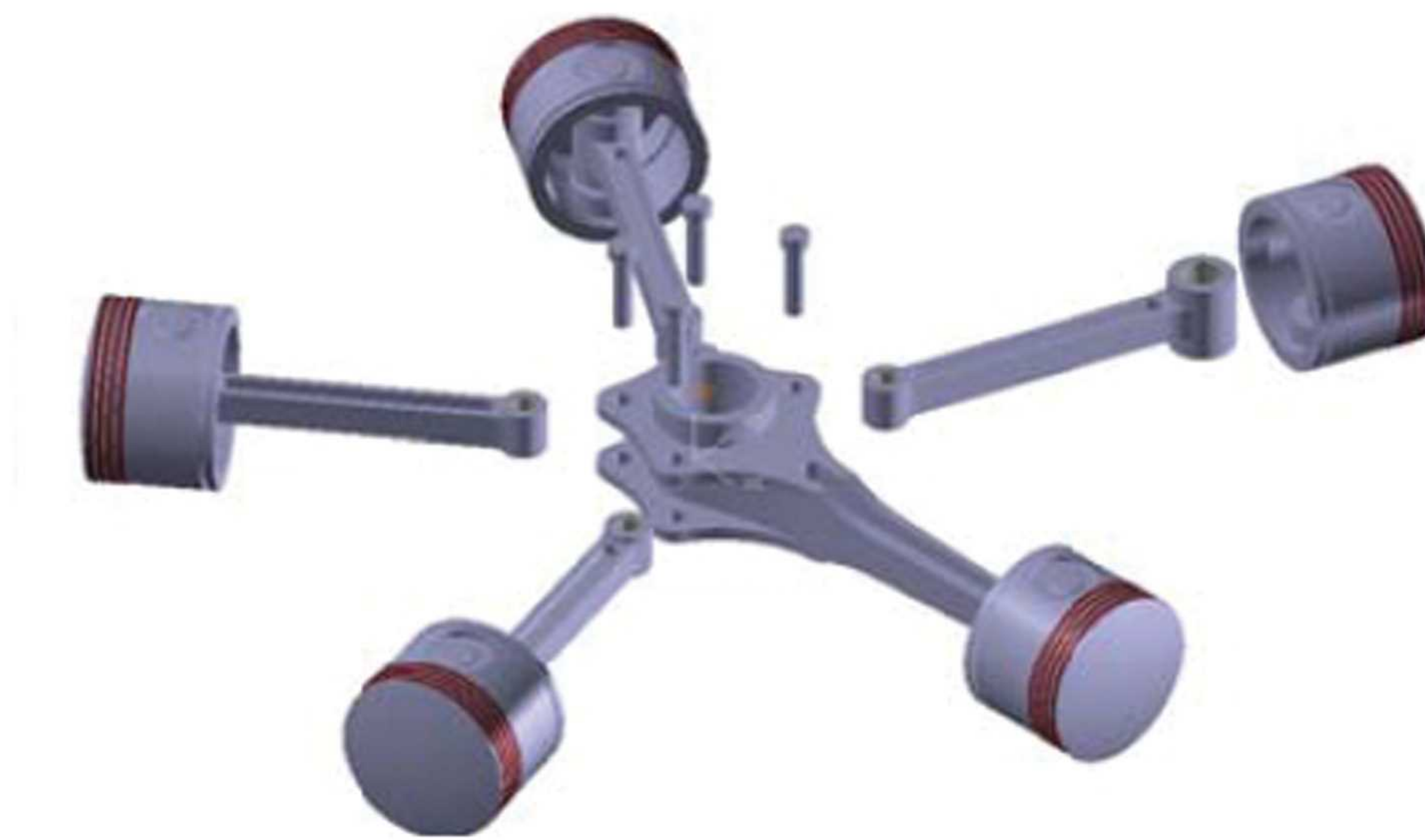
The exploded view of the Radial Engine assembly
